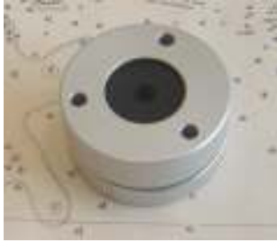
A cable deck gland that allows the cable with PL259 connector attached to pass through it.
